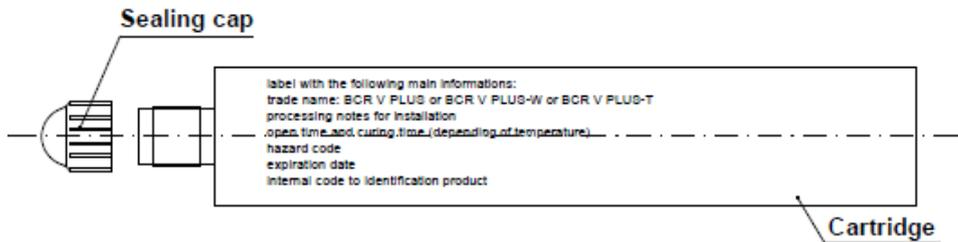
**coaxial peeler cartridge - size of 280 ml**
